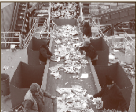
Pacific Rim sort line workers must remove any non-recyclable material from the paper "stream." Residents can make their work easier by putting only, paper, glass, metals and certain plastics in their carts.
